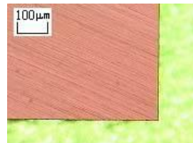
Die separation by back grinding
