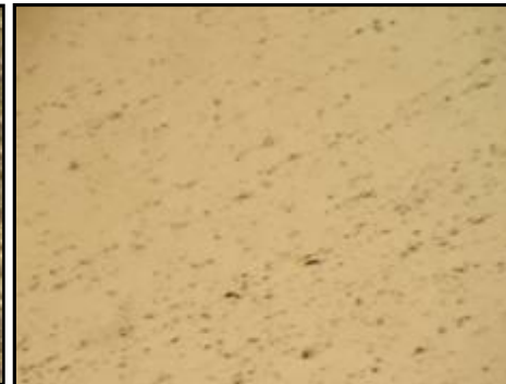
After 15 μm lapping
