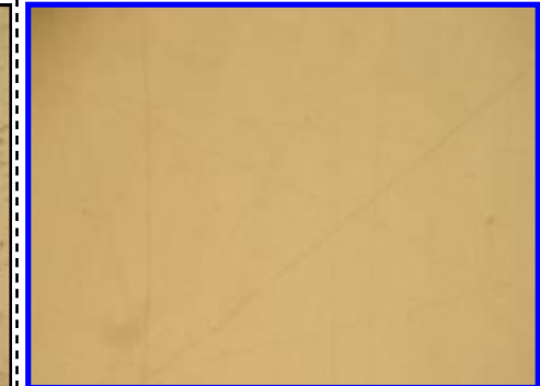
After 27 μm lapping
